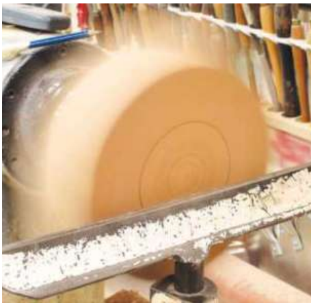
▲ Pic.4 Watch those fingers! The lathe speed is set at around 1,000rpm so anything finger-wise that you put over the toolrest is liable to be injured, so be careful!
